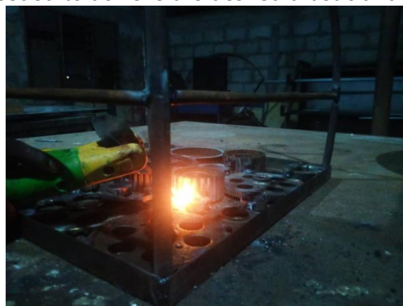
Figure 8: Welding process of the coffee table
