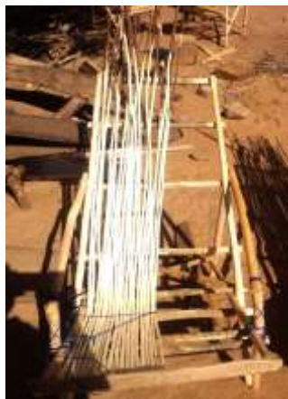
J. Twine-Weaving of Small Spokes onto the Skeleton
