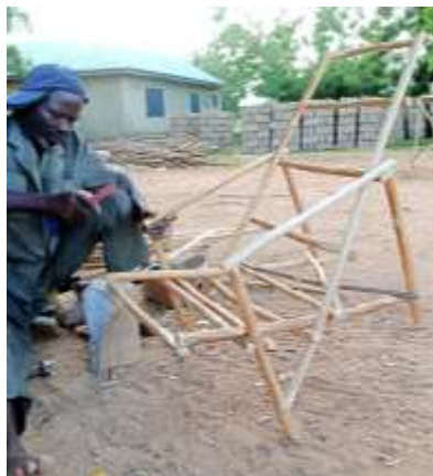
H. Finishing the Skeleton by Nailing all Seat Rails
