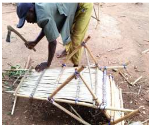
K. Trimming the Top of the Chair with a Carving Axe
