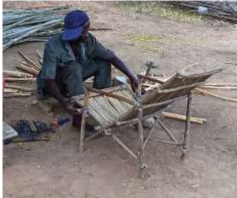
A. Measuring and Cutting of Stakes Using Old Furniture as a Guide
