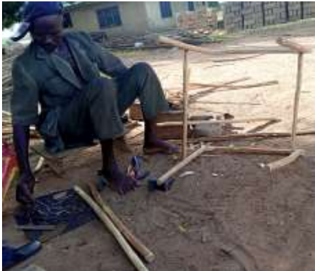
D. The Right and Left Arm Stands Nailed Together
