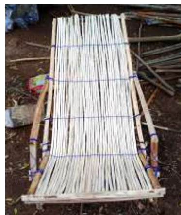
L. Trimmed and Ready for Top and Apron Rails Fining
