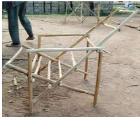
I. Completed Skeleton Ready for Weaving
