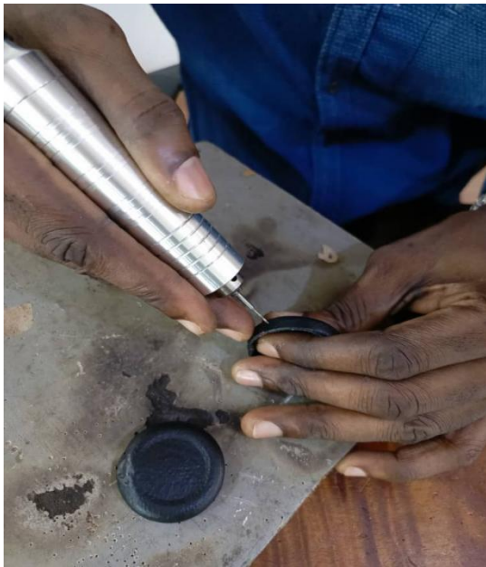
Figure 11: Perforating of holes
