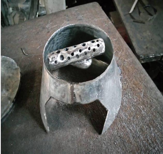
Figure 6: Construction of air duct of biomass Source: Researchers Own (2024)
