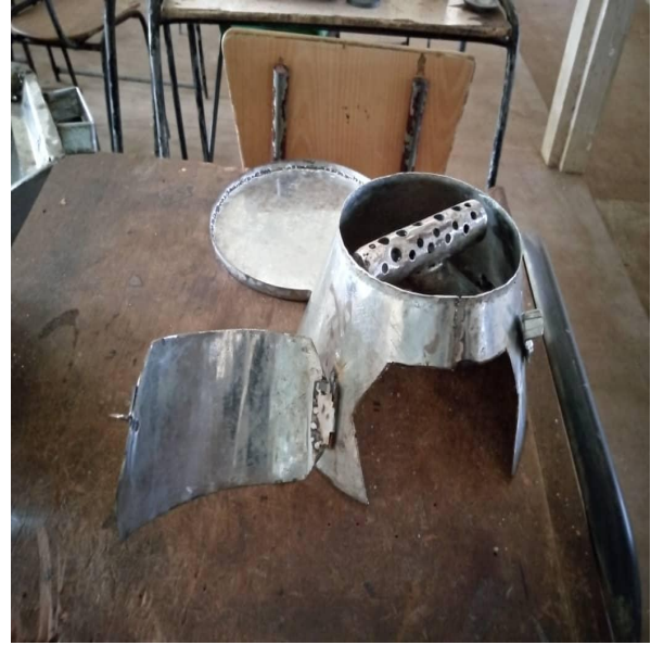
Figure 7: Construction of cover of air duct Source: Researchers Own (2024)
