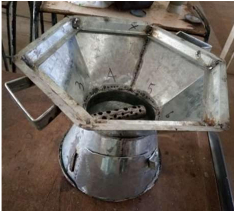
Figure 9: Finished Biomass Stove
