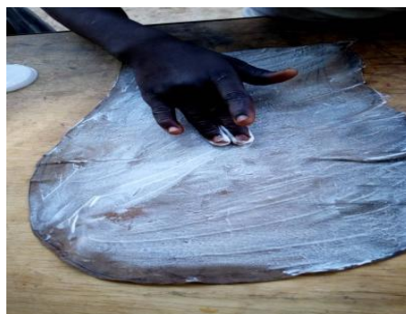
Figure 6: Spreading of PVA glue on the grain side of the leather. (Source: fieldwork, 2019)
