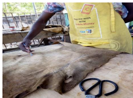
Figure 23: Tracing the template at the flesh side of the leather (Source: fieldwork, 2019)
