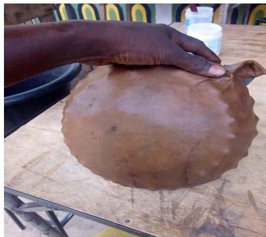
Figure 10: Pasting the final leather on the glued moulded leather (Source: fieldwork, 2019)
