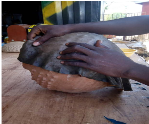
Figure 7: The first piece of leather placed on the pot during the moulding process (Source: fieldwork, 2019)
