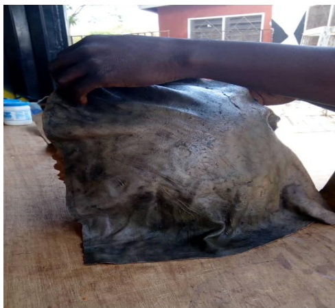
Figure 8: Overlapping the second and third layer of cased leather on the Bagadokor pot. (Source: fieldwork, 2019)
