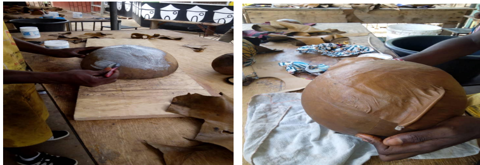
Figure 18: Spreading white glue and covering the overturn pattern with the last layer of leather
