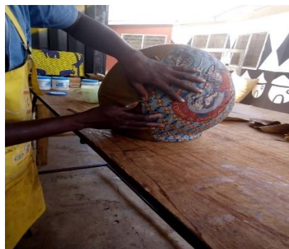
Figure 17: Reinforcing the five layers of leather with fabric and rubber
