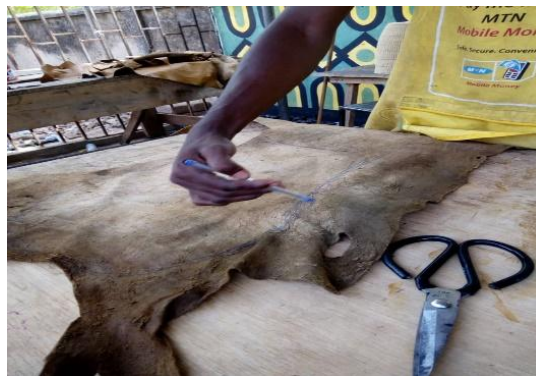
Figure 5: Tracing the template at the flesh side of the leather (Source: fieldwork, 2019)
