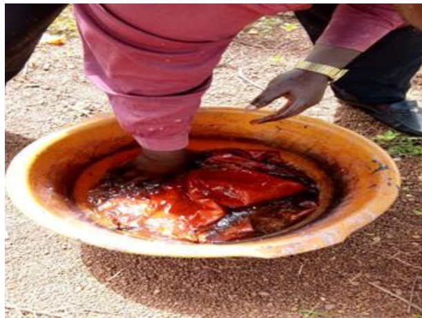
Figure 3: Soaking the vegetable tanned leather in a bucket of water (Source: fieldwork, 2019)
