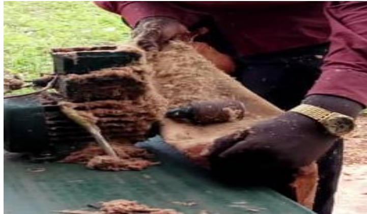
Figure 2: Sanding the flesh side of the vegetable tanned leather. (Source: fieldwork, 2019)
