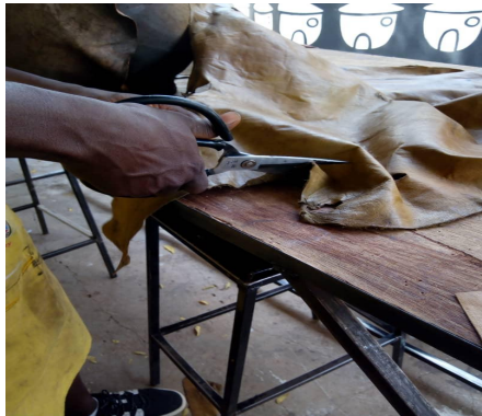
Figure 15: Cutting the various layers (5) of leather to serve as reinforcement.
