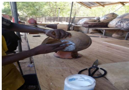
Figure 25: Applying white glue prior to laying the second set of leather layers (Source: fieldwork, 2019)
