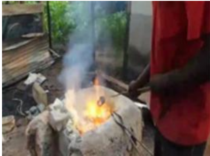
Figure 5: Melting and pouring of Metal ingots
