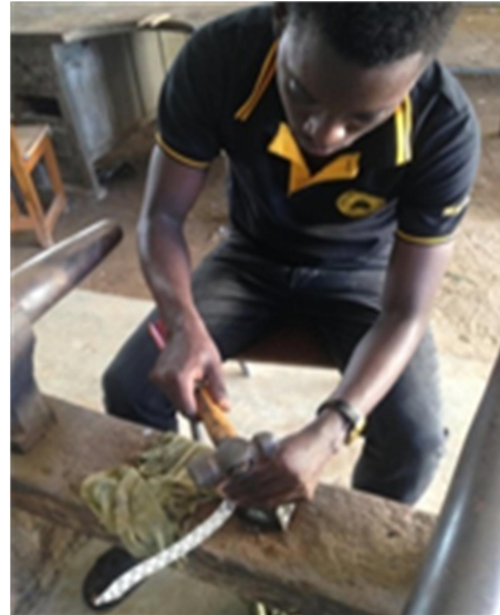
Figure 7: Doming of metal sheets.
